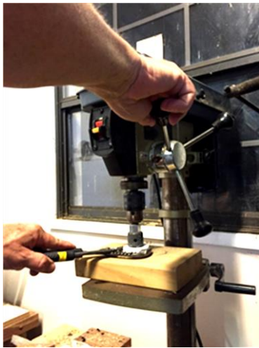
Figure 7: Drilling a 1" hole in the plastic endcaps.
