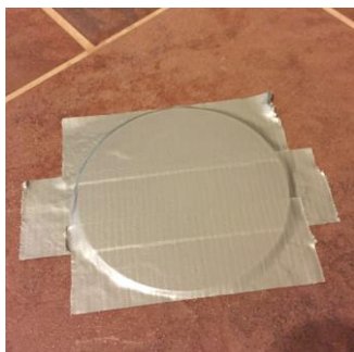
Figure 9a: Duct Tape used to remove CD Label
