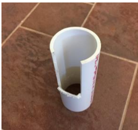
Figure 2b: Slot cut out of the PVC
