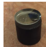
Figure 6c: Carefully glue concave lens to eyepiece tube.
