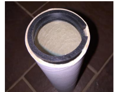
Figure 6b: Put Lens into tube followed with the final C-Ring on top.
