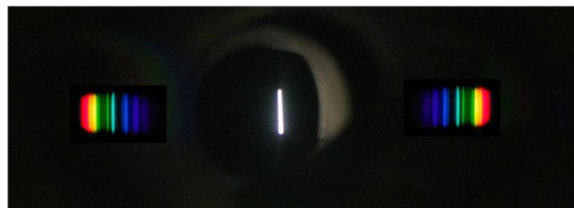
High Pressure Sodium Street Light
