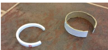
Figure 2d: Completed C-Rings. PVC on left, Cardboard on right.
