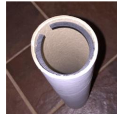
Figure 6a: Put a C-Ring into the tube.
