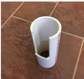
Figure 2b: Slot cut out of the PVC
