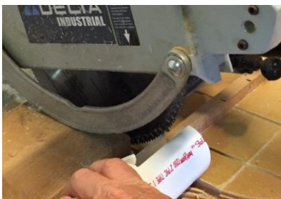
Figure 2c: Carefully cut C shaped rings from the PVC.
