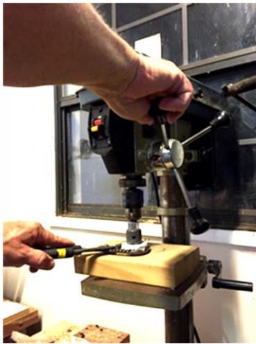
Figure 7: Drilling a 1" hole in the plastic endcaps.
