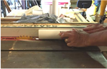
Figure 2a: Cut a slot in the 2" PVC pipe.
