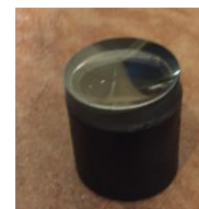
Figure 6c: Carefully glue concave lens to eyepiece tube.
