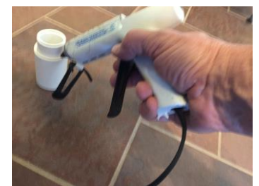
Figure 4: Assemble focuser and glue with hot melt glue.
